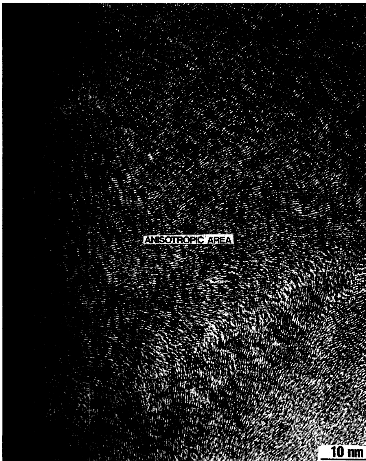
Fig. 5. P25 fibre cross-section. Lattice fringe TEM image. The comparison with Fig. 2 demonstrates the lower structural organization of P25 fibres relative to P55 fibres, while exhibiting similar textural features (anisotropic domains). Note the absence of interlayer decohesions.
