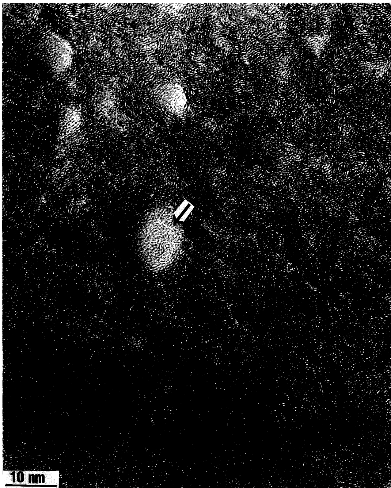
Fig. 7. T400H fibre cross-section. Bright field TEM image taken in the light-grey part of a fibre from Fig. 6. The presence of holes (arrow) attests that the area imaged is close to the fibre surface.
